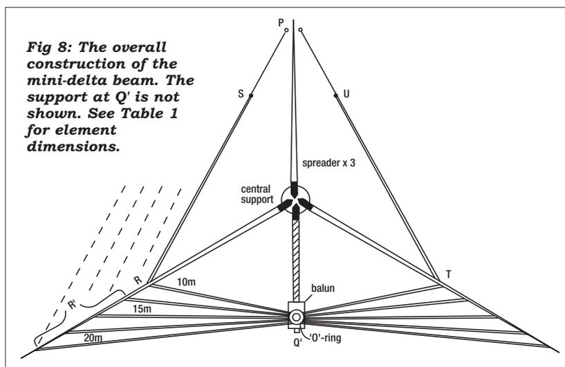
Fig 8: The overall construction of the mini-delta beam. The support at Q' is not shown. See Table 1 for element dimensions.
