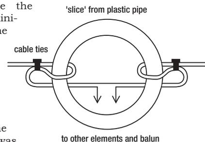
**Fig 6: The mid-point of the folded element.**
